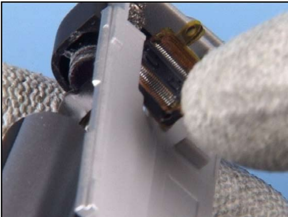
15. Carefully separate the C-COVER from the Upper Block and carefully slot the flex connector through the C-COVER. Always use a new C-COVER.
