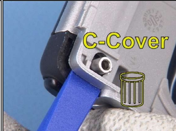
14. Loosen the C-COVER from the HINGE, also using the SS-93.
