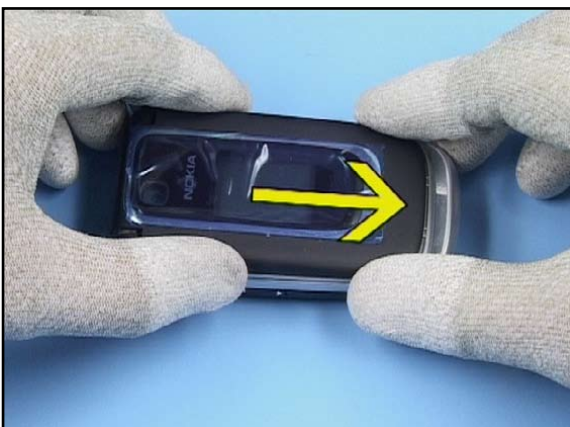
11. Put the A-COVER to the right guides first.
