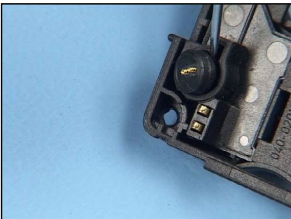
23. Ease out the MICROPHONE and remove it with tweezers. Do not touch the springs.
