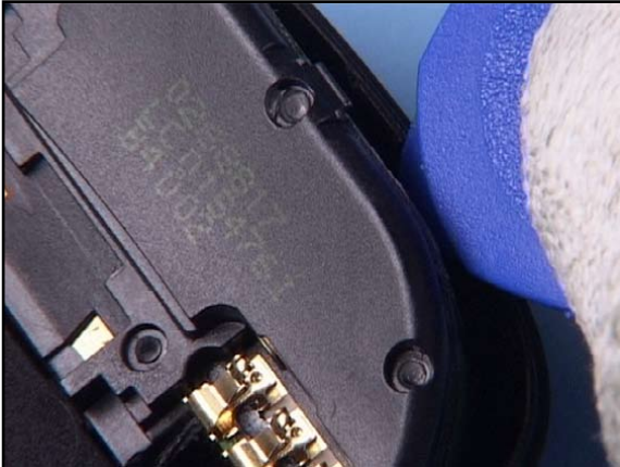
25. The ANTENNA ASSY can be released with the SRT-6 easily.
