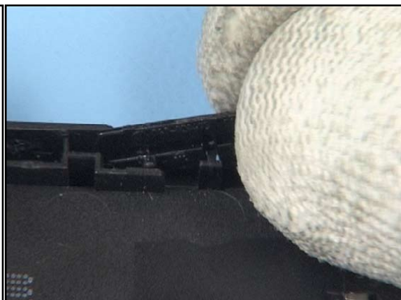
6. Insert the Buttons and lock them with your fingers.
