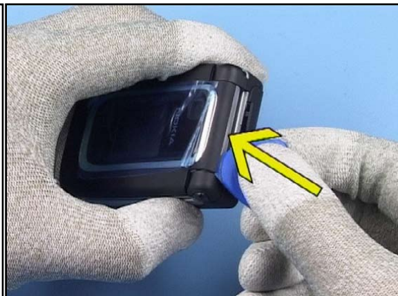
10. Now, shift along the SRT-6 to release the underneath snaps.
