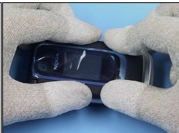
12. Then press down and lock the other underneath snaps.
