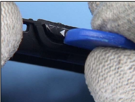
21. Release all buttons with the SRT-6 as shown.
