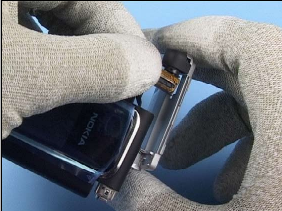
13. Slot the flex connector through the D-COVER with caution.
