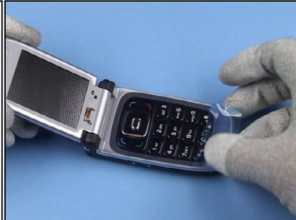
8. Protect the inner side of the lower block.
