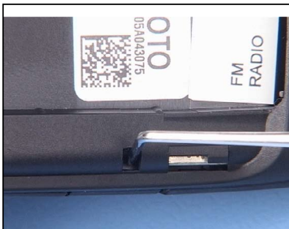
9. Use the dental pick to unlock the clips at both sides.
