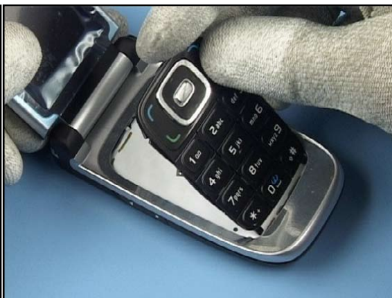
24. Finally, assemble the KEYMAT, starting from the lower side.
