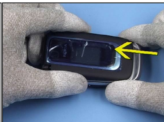
12. Now, remove the A-COVER by sliding it around 4mm to the shown direction and then lift it up.
