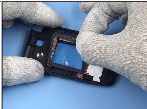
10. Put the Front DISPLAY GASKET to the A-COVER. Pay attention that all guiding pins fit to the gasket. Check also proper position of the CAMERA GASKET.
