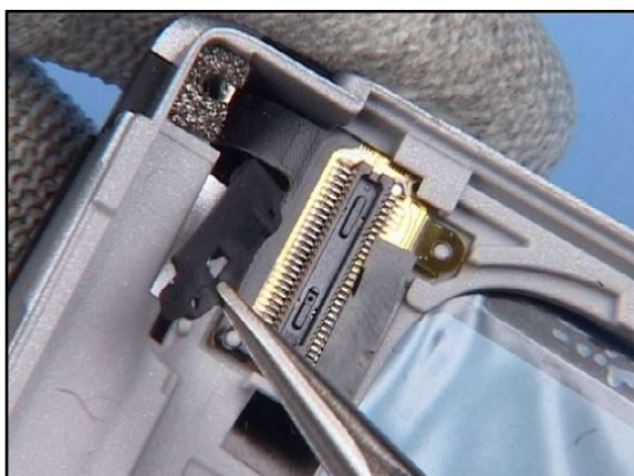
11. Remove the MIC-RUBBER with tweezers.
