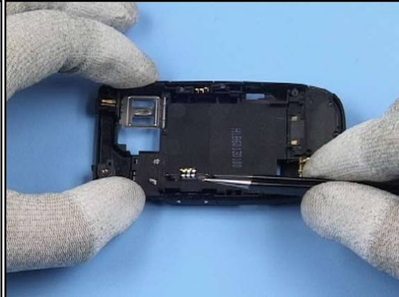
20. Remove the VOLUME KEY and on the opposite side the FUNCTION/POWER KEY with tweezers. Take care not to bend the springs.
