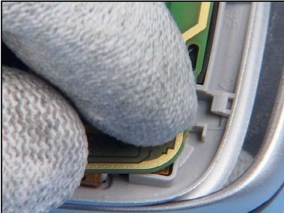
7. Properly lock the LCD connector.
