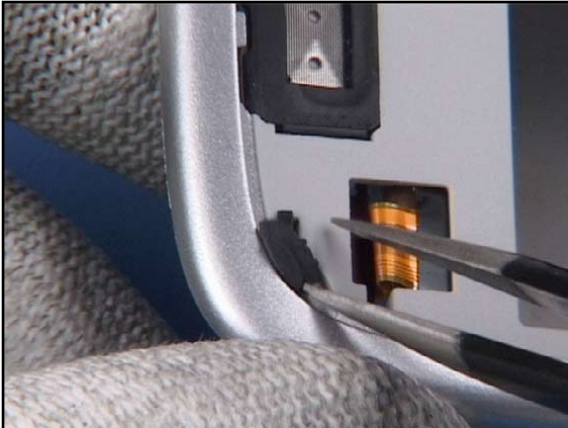
7. Remove both RUBBER STOPPERS with tweezers.
