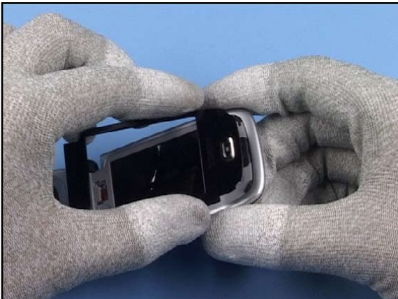
15. Exactly position the DISPLAY BEZEL. Start on the top (earpiece section) by sliding in the bezels' hooks to the B-COVER, press gently all over the bezel to ensure that whole part adhere properly.
