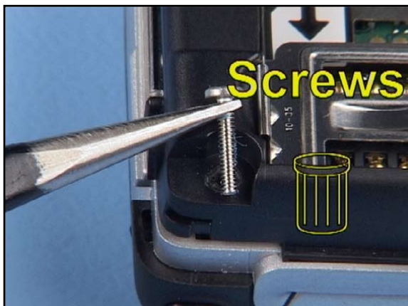
7. These screws are covered with locking compound and can't be reused again.
