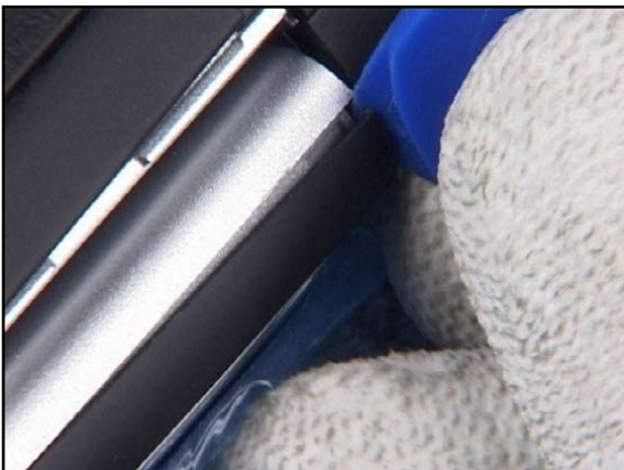
9. Gently unlock the A-COVER from the backside.
