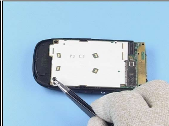
10. Insert the board screw with tweezers.
