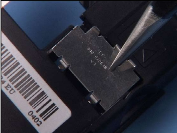
1. Insert the BATTERY SPRING and click it into its place.
