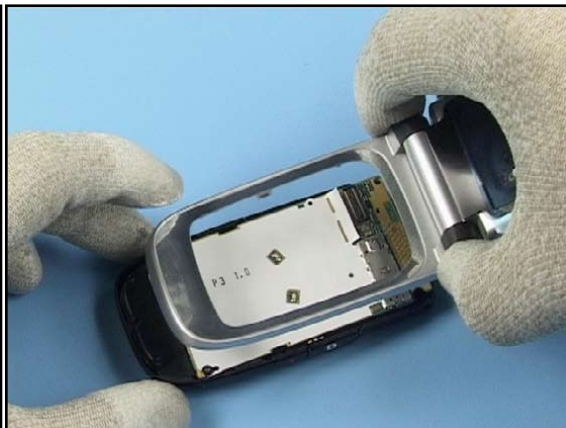
20. Open B-COVER by pressing the release button, then mount the C-COVER with the Upper Block onto the D-COVER.
