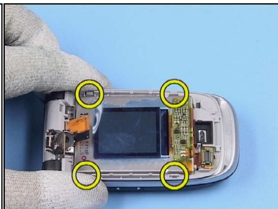
18. Unlock the four clips which hold the NAPA DISPLAY MAIN.
