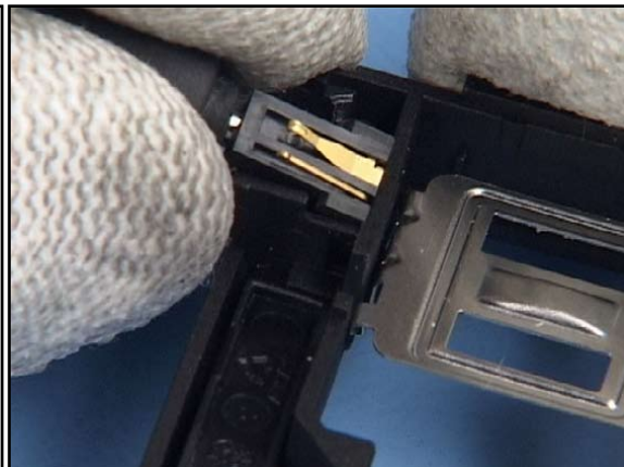
22. Remove the DC JACK with the DC Plug.
