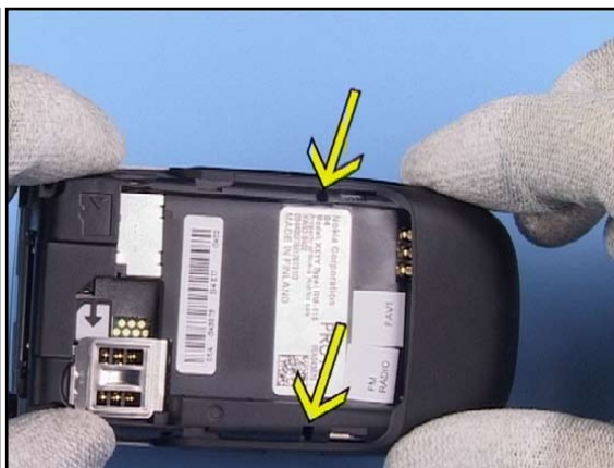
8. Hold the assembly as shown. Locate the 2 holes in the D-COVER.
