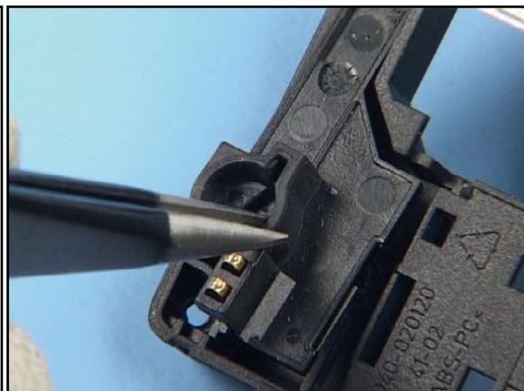
24. Remove the BLUETOOTH ANTENNA with tweezers.
