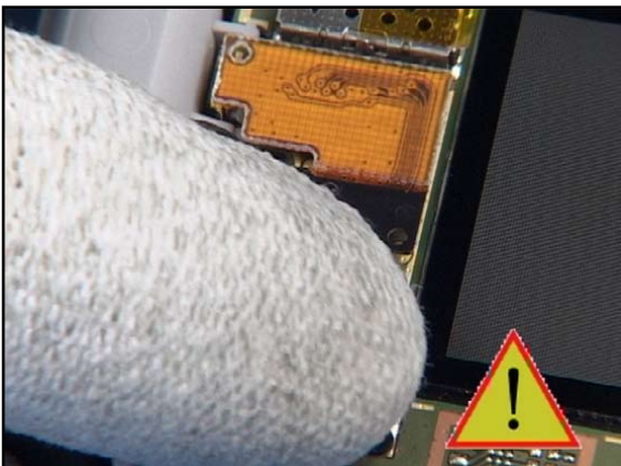
9. Carefully close the two flex connectors without touching the CAMERA.
