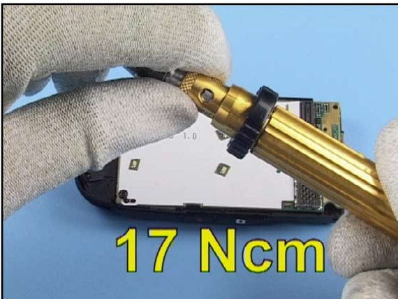
11. Set the correct torque and tighten in.
